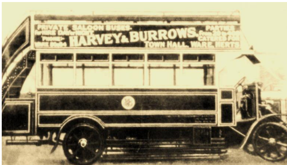
A side view of one of Harvey and Burrows open top double deckers. It was quite common in the early 1920s for such buses to have solid rubber tyres and the driver exposed to the elements due to an open cab with no windscreen provided. The firm ran small single decker buses on the more rural routes unsuited to larger buses. In addition they also provided vehicles with driver for private hire work.
