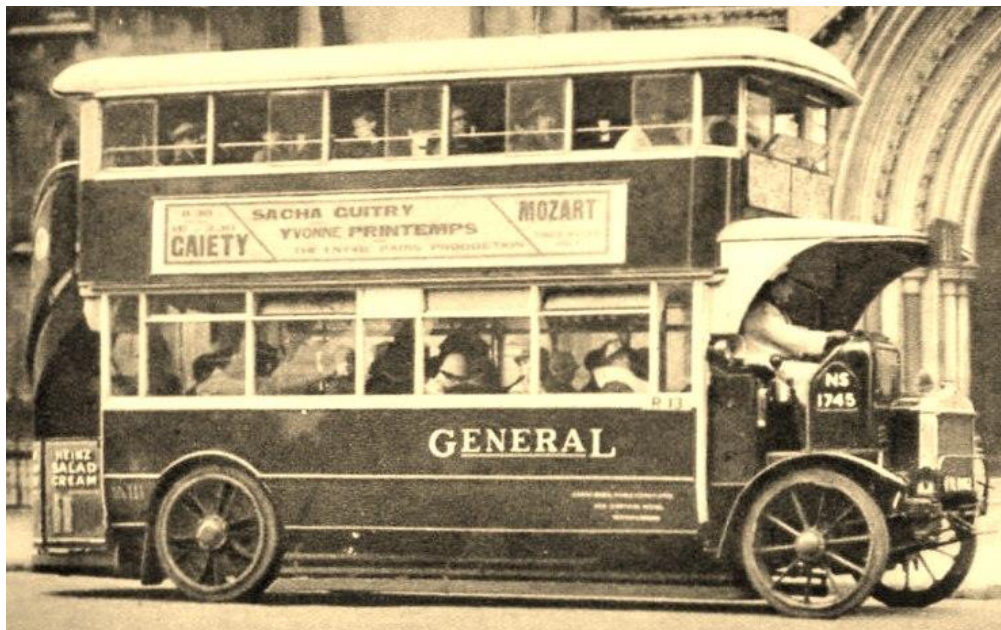
As time progressed the double deck buses were improved to varying degrees. This one has windows and a roof for upstairs passengers but the driver remains out in the cold. This type saw use on services in Hertfordshire including the 310 to Hertford.
