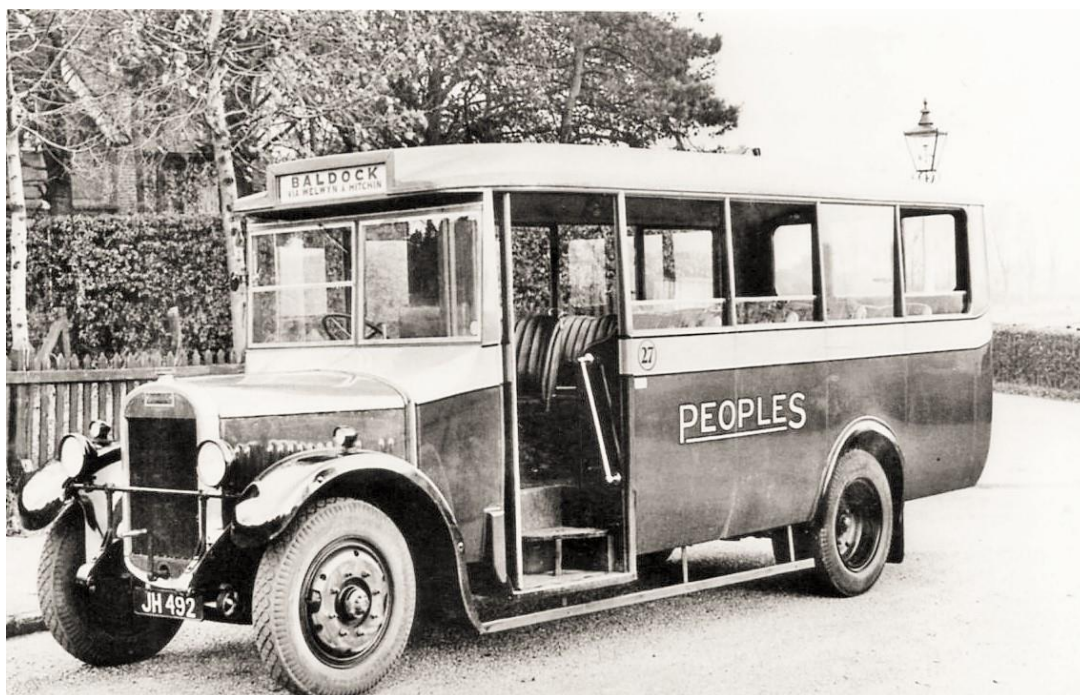
A typical single deck bus operated by The People's Buses from their Ware Garage. These buses had pneumatic tyres and were more comfortable and pleasant to ride in than many of the buses provided on the National run services. These smaller buses usually carried less than 20 passengers because above that number the law required a conductor.
