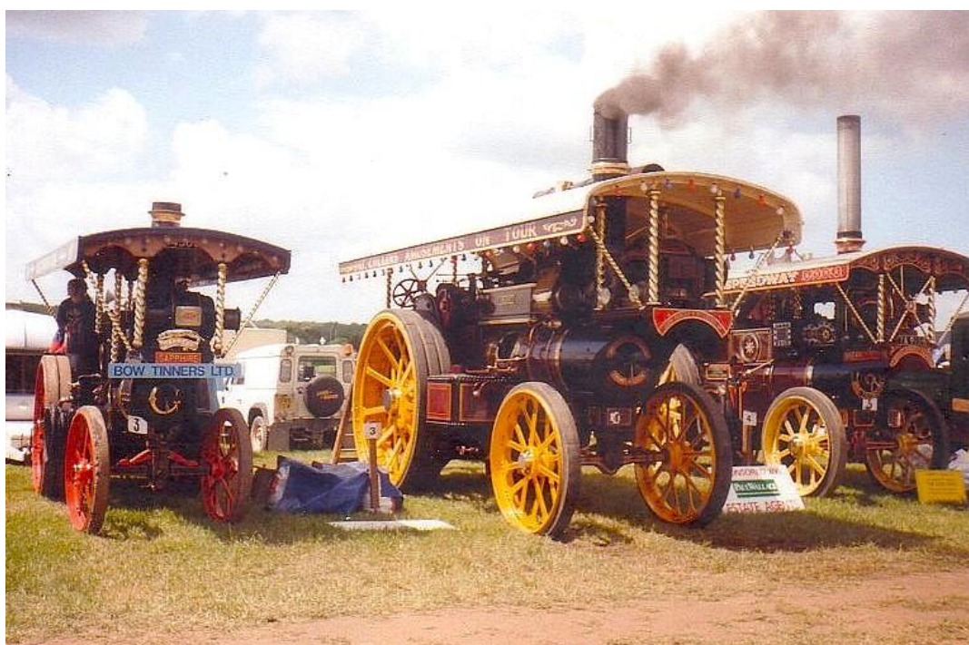
Showman's traction engines being prepared for venturing out into the main ring later in the day. The two engines on the right are using their longer extension chimneys which help with pulling the air through the fire to raise steam pressure as well as keeping the smoke away from the spectators.
